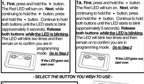
While the LED is on, press the button you wish to use. (If your block has 8 switches press the + button, if not, press any button you'd like to use). The LED will blink off once and then remain on.
